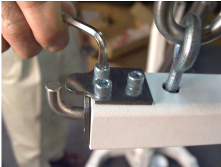
Remove outer 2 Screws Loosen inner Screw
