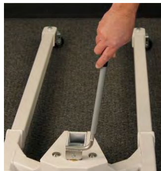
Install Handle Extension
