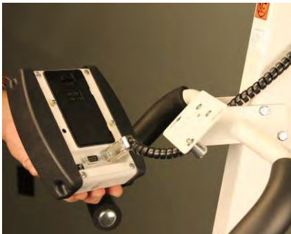
Install load cell cable and secure with cable connector retaining screws
