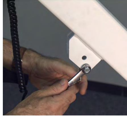
Remove Bolt, Washer & Nut
