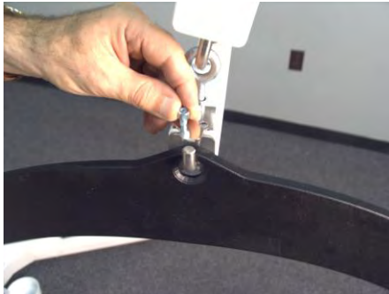
Lift hoop slightly to ease screw installation
