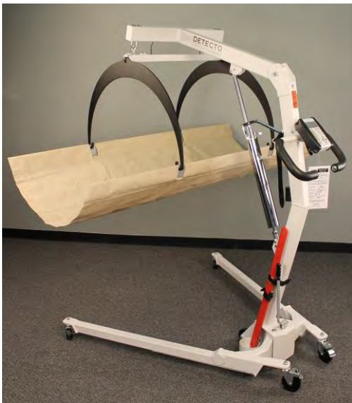
Attach stretcher to hooked ends of support bars
