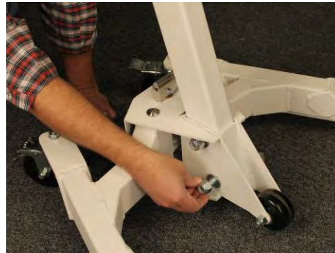
Install Bolts, Washers & Nuts
