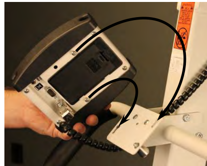
Align screw heads with large end of slotted holes and pull down to secure indicator
