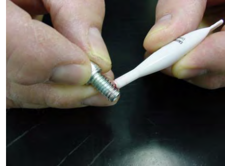
Apply a small amount of Loctite® to screw threads
