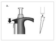
Hold the pipette shaft over a suitable disposal bin and press the tip ejection button all the way down.
