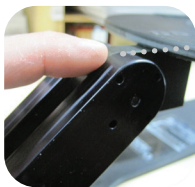
Step 1 - Lock the platform cam
