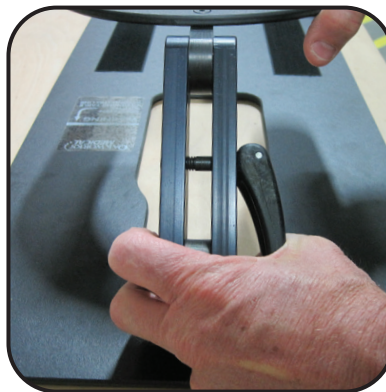
Step 5 - Close cam to the final position.
