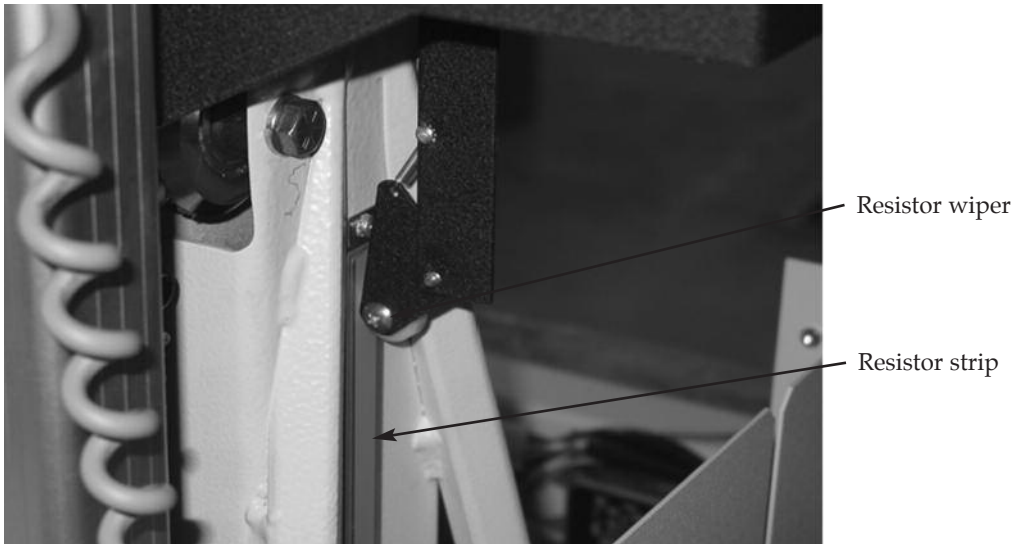
Figure 10.1. Height position sensing resistor strip
