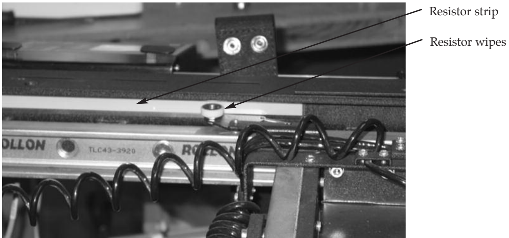
Figure 10.4. X position sensing resistor strip (tabletop removed for viewing)
