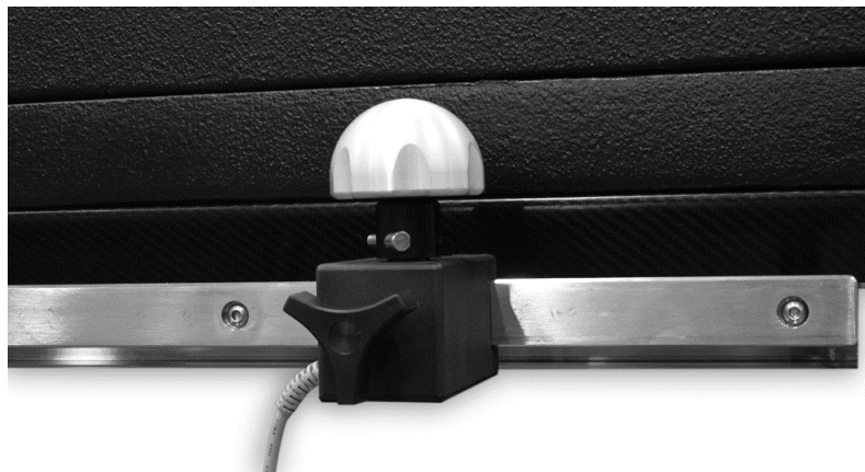
Figure 2.6. Push button (on handle) releases tabletop for free-float X-Y motion.
