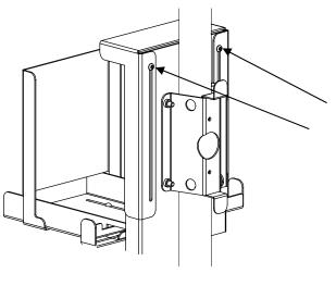
Use the provided security screw wrench to loosen the Top Cover of the CPU Holder
