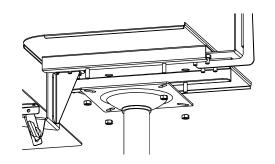
Place the Top Assembly on top of the Column Assembly and fasten in place with the provided nuts.
