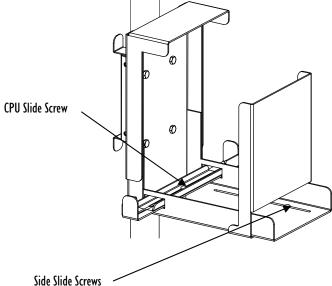
Remove the CPU Slide screw and insert the CPU slides into the base as shown with the smaller on top. Reinsert the screw loosely. Loosen the screws holding the side slide in place. Place your CPU on the base and position the slides closely around it. Remove the CPU and tighten the slide screws. Replace the CPU and secure it in by retightening the Top Cover.
