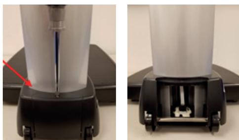
1. Using a Phillips screwdriver, remove the door at the back of the platform base.
