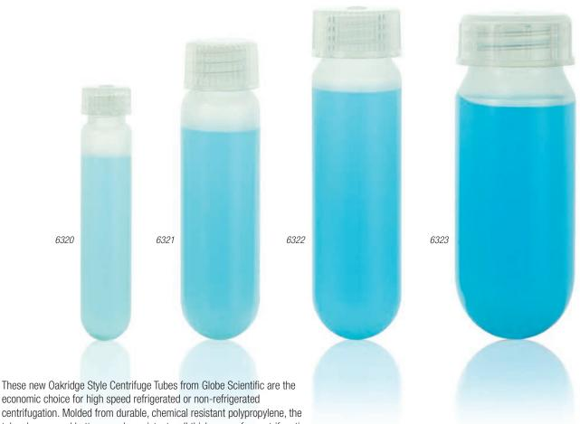
economic choice for high speed refrigerated or non-refrigerated centrifugation. Molded from durable, chemical resistant polypropylene, the tubes have round bottoms and consistent wall thicknesses for centrifugation at up to 50,000g when filled to 80% of their nominal capacity. Oakridge style tubes are autoclavable and re-usable and are designed with leakproof linerless closures.
