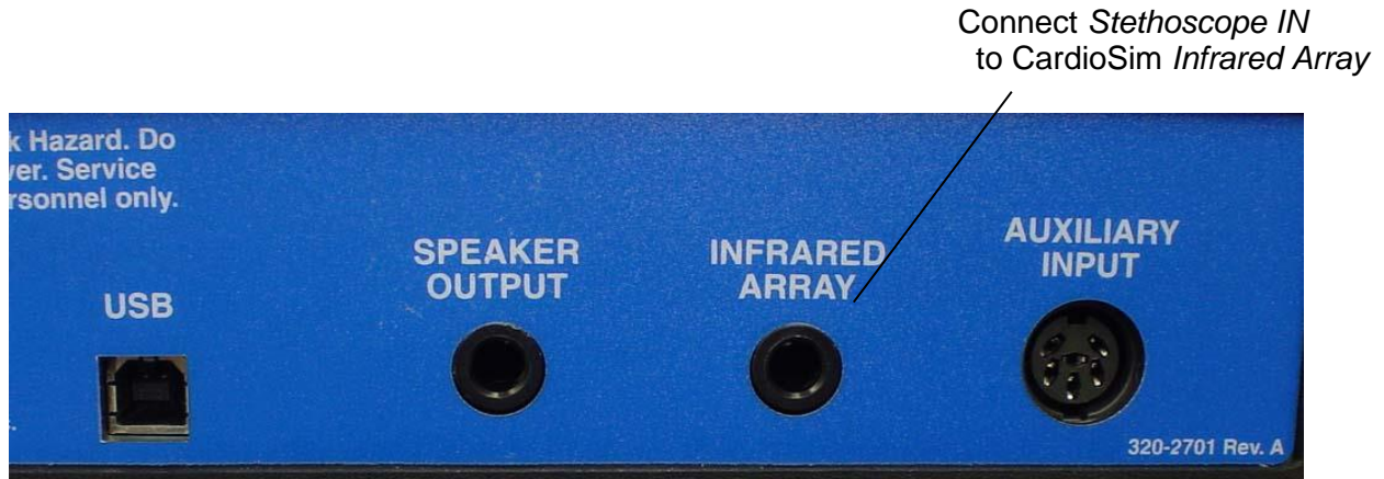
Figure 12 Connecting SimulScope to CardioSim
