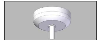
Push cover and end ring over the ceiling bracket and tighten them (0.5Nm)
