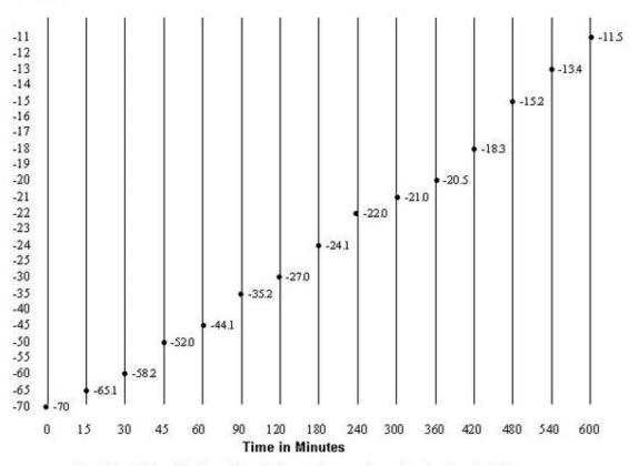
Graph is of Biocooler Cryo placed at room temperature after freezing for 24 hours. Temperature of samples in interior holes were then monitored with a digital thermometer.
