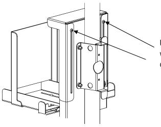
Use the provided security screw wrench to loosen the Top Cover off the CPU Holder
