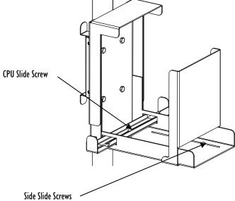
Loosen the CPU Slide screw and adjust the width of the slides to match your PC. Loosen the screws holding the side slide in place. Place your CPU on the base and position the slides closely around it. Remove the CPU and tighten the slide screws. Replace the CPU and secure it in by retightening the Top Cover.
