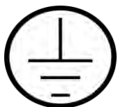
Protective Earth Ground Symbol
